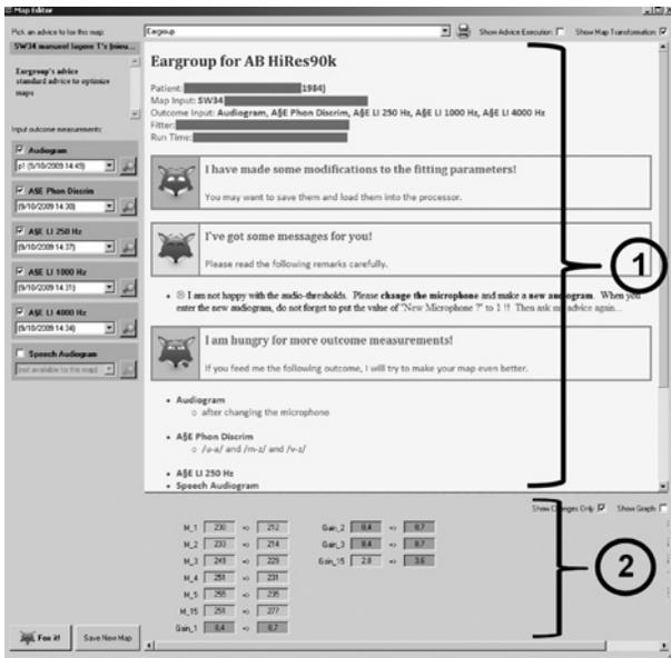
**FIG. 3.** A typical response from FOX, after input of outcome data, is illustrated in this screen shot. The output consists of messages (1) and suggested modifications of the MAP settings (2). See text for further details.
