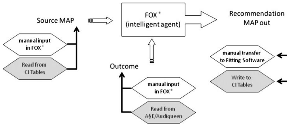
**FIG. 1.** Fitting to Outcomes eXpert working principle. An initial program and various psychoacoustic test results may be input into FOX, which then delivers fitting recommendations as output. *Shaded boxes* illustrate function when interfaced with proprietary outcome and CI fitting software, whereas *unfilled boxes* denote stand-alone function.
